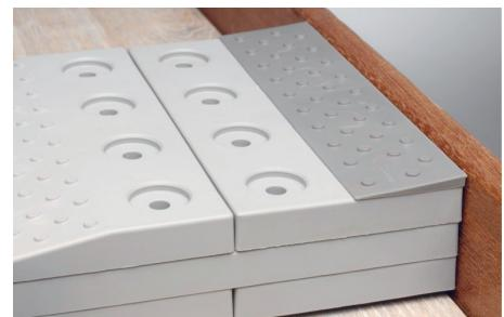
Rotate the half-size fitting plate 90 degrees and place it onto a plate part. Attach it with a firm tap of the hammer (always use the strike plate). Determine where you may have to shorten the fitting plate based on the best fitting height. Cutting lines are present on the plate for this.
