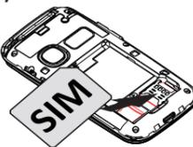
**Note!** This device accepts micro SIM or 3FF SIM card. Use of incompatible SIM cards may damage the card or the device, and may corrupt data stored on the card.
