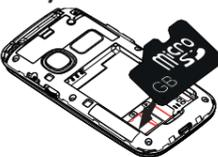
**Note!** The circuit boards (metal part) on the cards must not be scratched or bent. Try not to touch the circuits with your fingers. Use only compatible memory cards with this device. Compatible card type: microSD, microSDHC. Incompatible cards may damage the card itself, the device and corrupt any data stored on the card.
