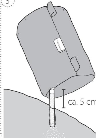
Hold the refill package with the tube facing up and insert the tube until approximately 5 cm into the refill opening of the inlet (meaning approx. 14 cm of the tube has to be inserted into the inlet). If the tube is not inserted deeply enough you will possibly not be able to refill the inlet. Now hold up the refill package for making the micro-beads flow into the inlet.
